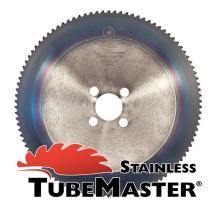
The TubeMaster Stainless saw blade has specifically been developed for cutting stainless steel tubes on orbital flying cut-off units. These saw blades can cope with cutting speeds between 60 - 120 m/min. TubeMaster Stainless offers high uptime due to a blade life up to  $3,5\text{m}^2$ , combined with high cut quality and production output.
